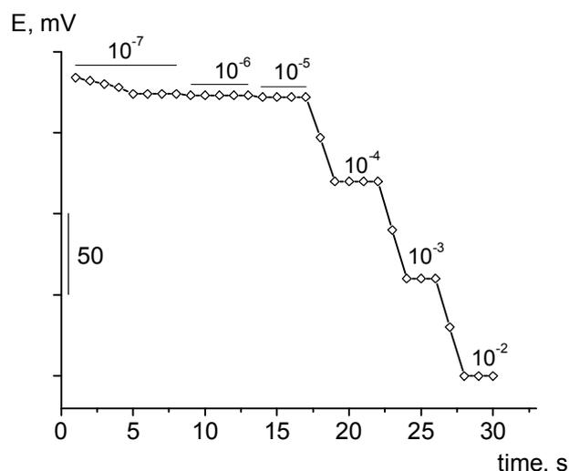
Fig. 2. Response time of diclofenac selective electrode.
