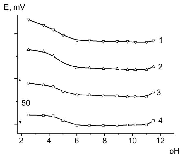
Fig. 3. Effect of the pH of test solution on the potential response of the diclofenac ion-selective electrode (1 – pC 3.3; 2 – pC 3.0; 3 – pC 2.3; 4 – pC 2.0)
